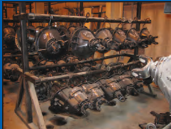
Rebuilt Rear Ends
