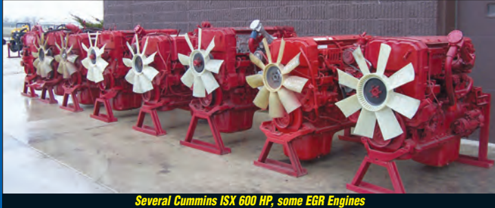
Several Cummins ISX 600 HP, some EGR Engines
