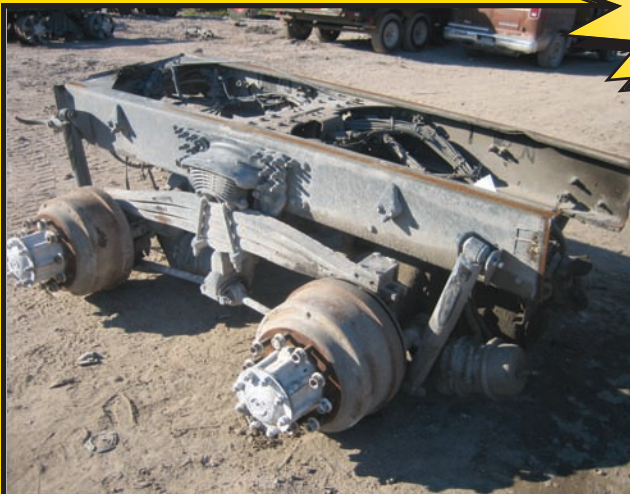
Rockwell Rd 23160 4.32 46,000 LB Volvo T-Ride Susp. Pilot Hubs
