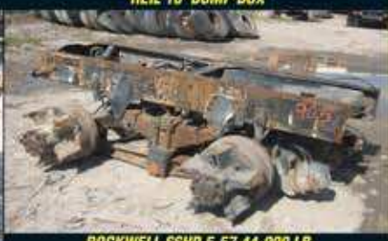
ROCKWELL SSHD 5.57 44,000 LB HENDRICKSON SUSPENSION
