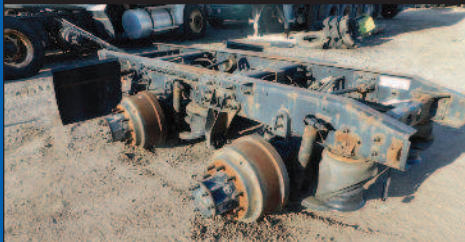
CUTOFF 2012 INTERNATIONAL PROSTAR MERITOR MT40-14X 3.36 RATIO 40,000LB
