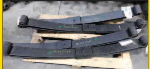
NEW 12K FRONT CHASSIS SPRING TAPER LEAF W/RUBBER BUSHING FITS: INTERNATIONAL 7600 SEVERE TRUCKS (BUILT ON 04/01/2002 & LATER) PART # 3712717C92
