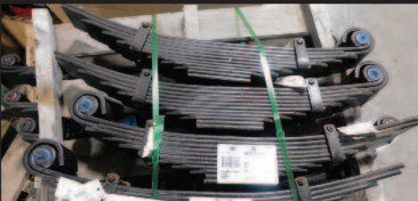
NEW REAR SPRING ASSEMBLY FITS INTERNATIONAL 4900 4X4 PART # H45031000
