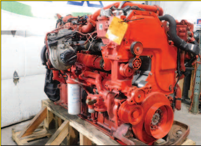
2015 CUMMINS ISX-15 CM2350 600 HP CPL 3939 MILEAGE 116,796
