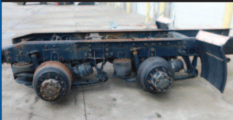
MERITOR 40K REAR AIR RIDE CUT OFF WITH MT-40-14X DIFFS WITH 3.36 RATIO MILEAGE: N/A
