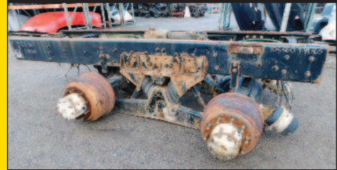
CUTOFF 2000 STERLING VIN#:2FZNRJBB2YAA94095 MERITOR 6.43 RATIO WITH LOCKERS
