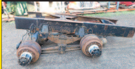
Heavy Spec Rear Cutoff Hendrickson with 3.55 ratio
