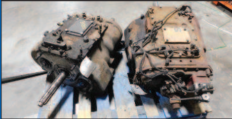
EATON FULLER TRANSMISSION RT0-16910B-DM2 MILEAGE 508,255 AND MODEL FRMF-15210B MILEAGE N/A
